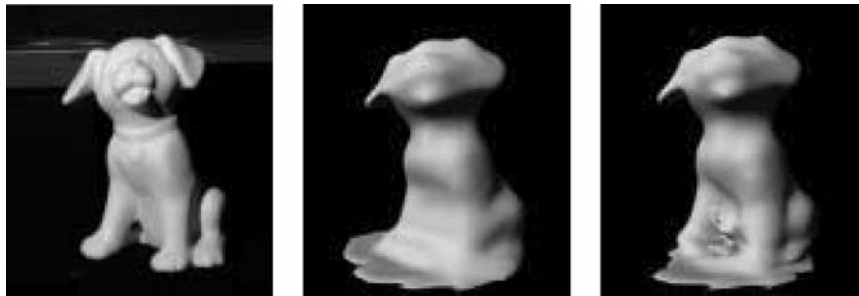
Figure 32. Left: Captured image of the dog. Center: Results of space carving. Right: Results of shadow carving with 4 lights and 24 views.
