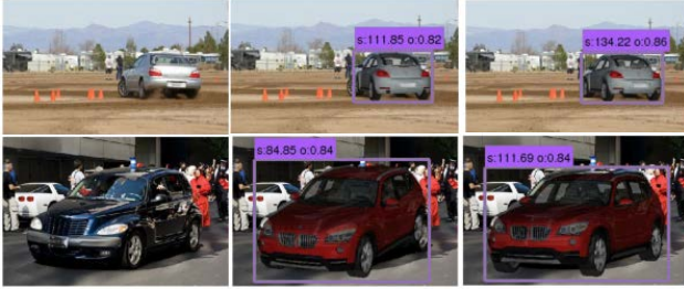
Figure 8: Effect of fine tuning. (left) original image, (middle) initial detection, (right) continuous fine tuning using Single-Component Metropolis Hastings
