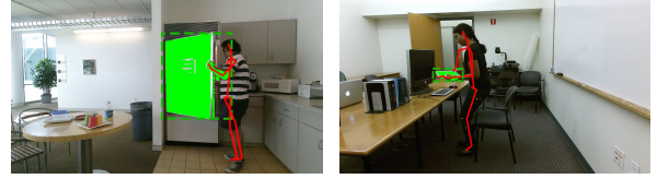
Figure 3: Examples of the human skeletons (red line) and the extracted interactive objects (green mask, left: fridge, right: book).
