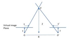
Figure 2: Rectified Stereo Rig (B is not the mid point of OO', the figure isn't symmetric)
