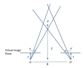
Figure 3: Rectified Stereo Rig with image plane error
